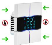
For installing or removing the faceplate, please be careful that only pushes corners. Do not push the side middle, it may damage this product. Look at the picture, green arrow shows that there must be a push out for removal or push in for install.
